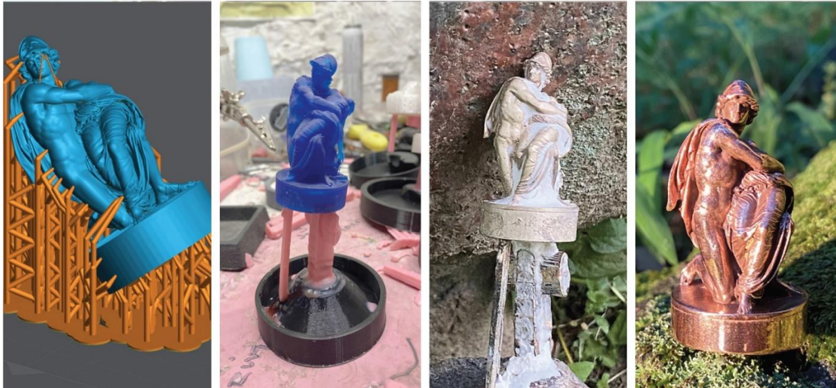
Images of the 3D-printing and casting process from left to right: 1) Casting model in Lychee Pro with supports. 2) Printed model with Liqcreate Wax Castable resin attached to the wax sprue. 3) Bronze cast, quenched and ready for cleaning. 4) Bronze casting prepared for final polishing.
