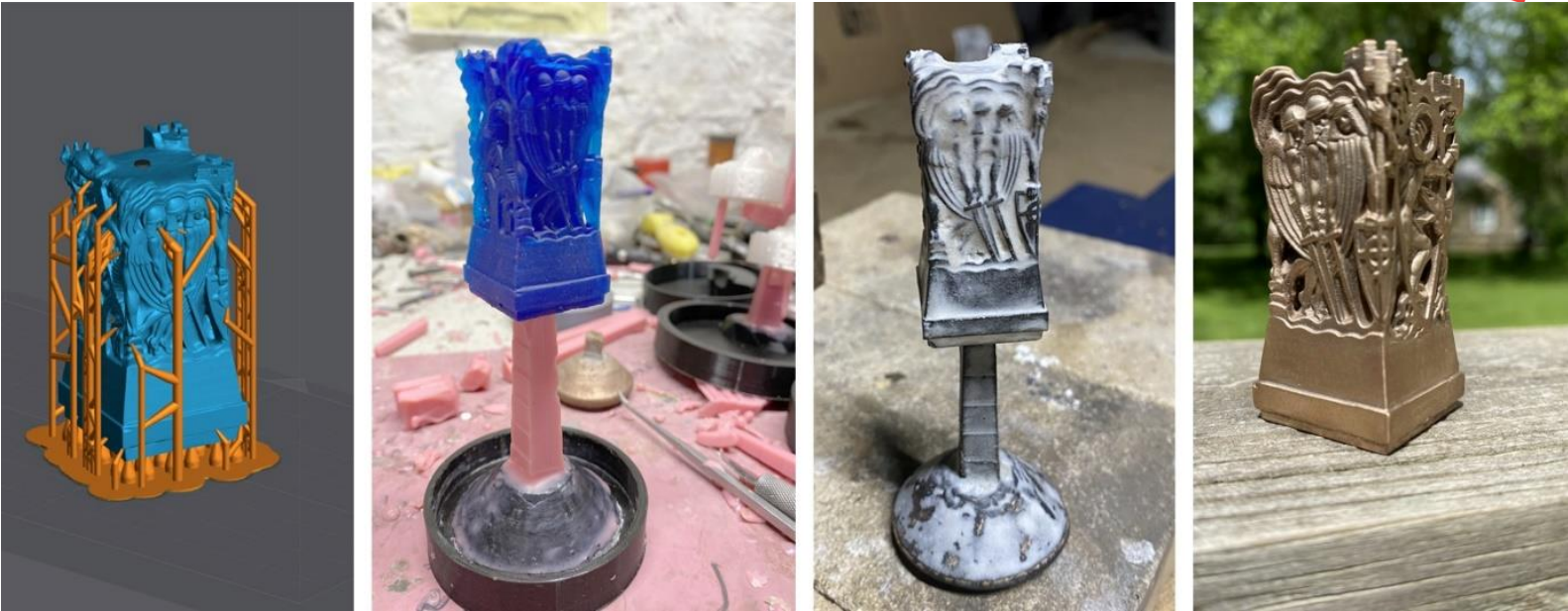
Images of the 3D-printing and casting process from left to right: 1) Casting model in Lychee Pro with supports. 2) Printed model with Liqcreate Wax Castable resin attached to the wax sprue. 3) Bronze cast, quenched and ready for cleaning. 4) Bronze casting prepared for final polishing.
