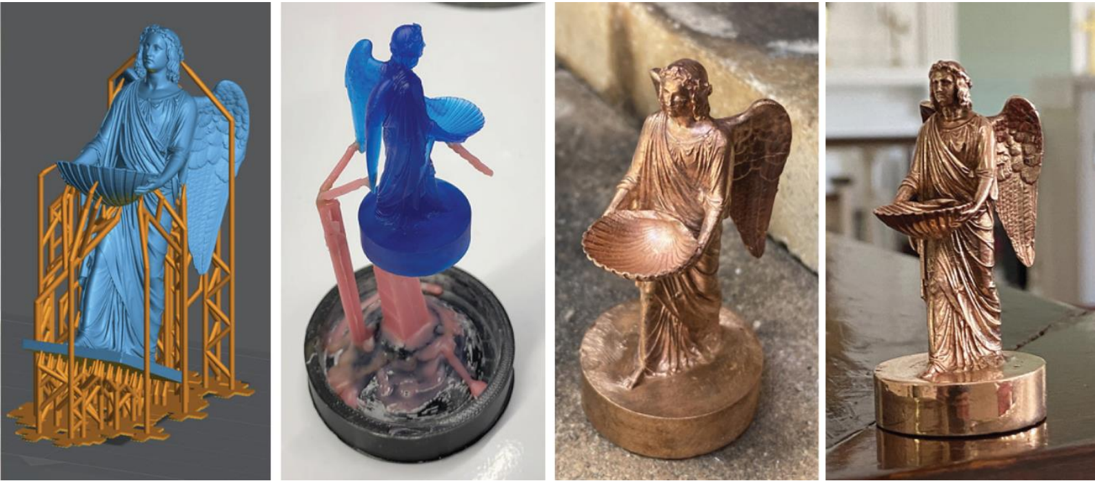
Images of the 3D-printing and casting process from left to right: 1) Model in Lychee Pro with supports. 2) Printed model with Liqcreate Wax Castable resin attached to the wax sprue. 3) Bronze cast, quenched and ready for cleaning. 4) Bronze casting prepared for final polishing.
