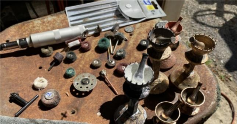
Image: preparations for finishing bronze parts cast with Liqcreate Wax Castable resin.
