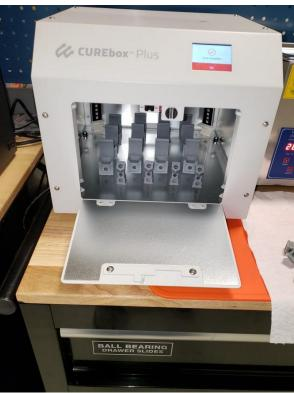
Image: printing parts in the <u>Epax3D X10</u> and post-curing engineering resin <u>Liqcreate Strong-X</u> in the <u>Wicked Engineering Curebox</u>.
