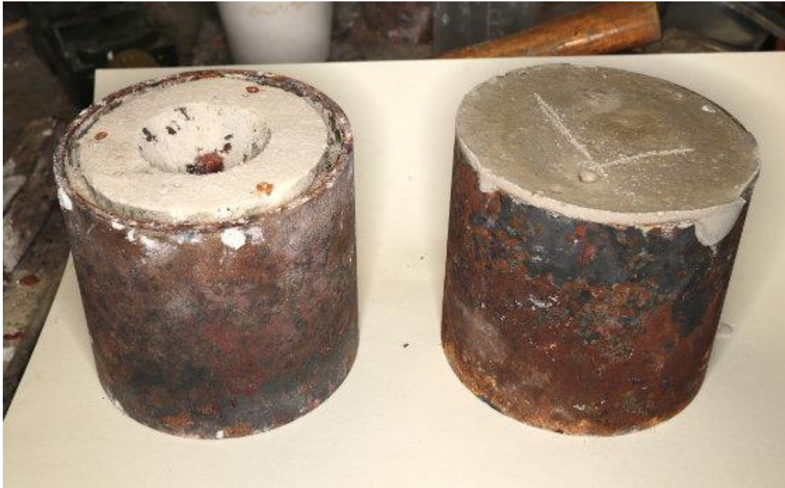
Image: photo of the casting of the cylinders without passing through a vacuum.
