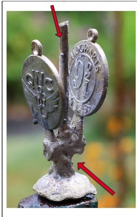
Images left and right are the raw result after quick casting. Photo in the center are the casting tip without vents for some parts.
