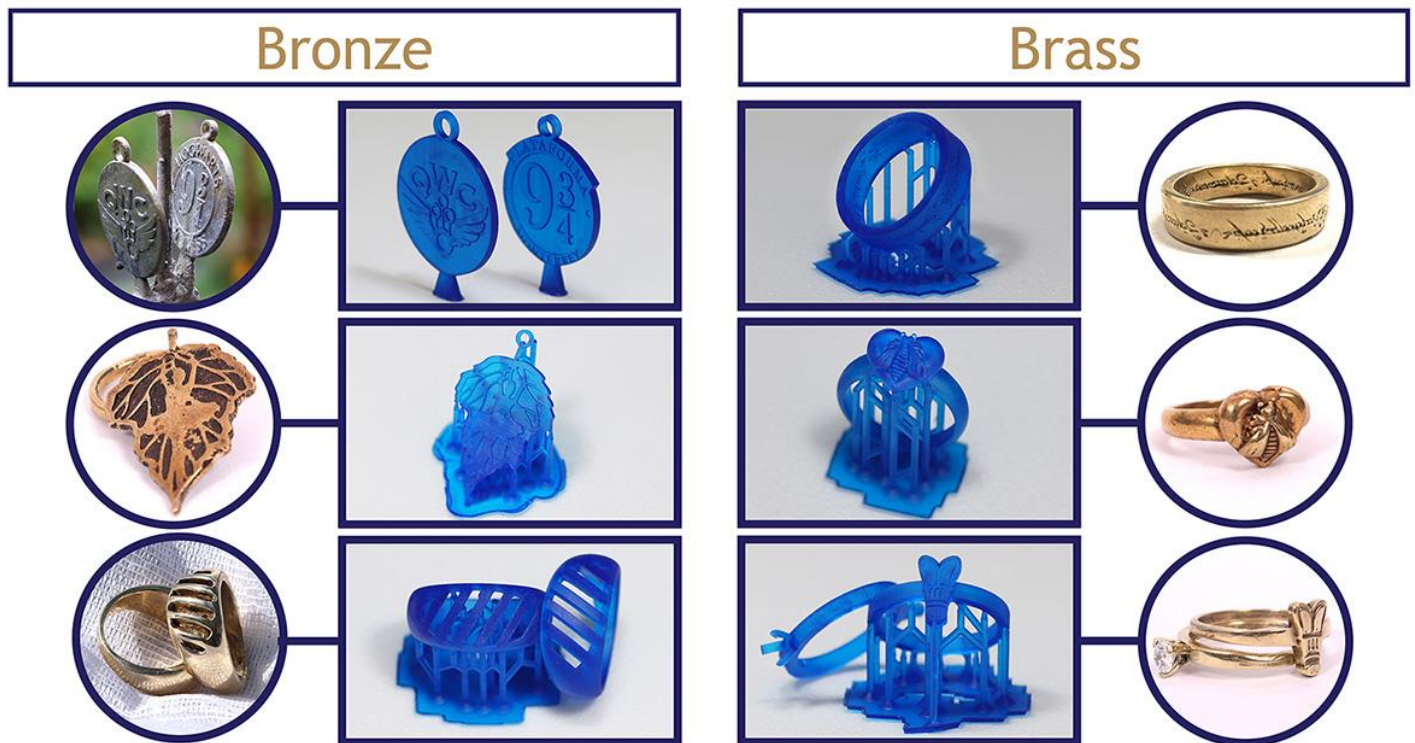
Image: different applications casted with Liqcreate Wax Castable resin, ideal for jewelry applications.
