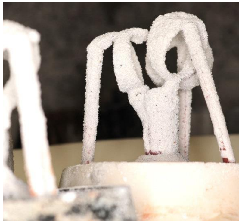
Image: The assembly of the elements on the casting axis with the vents and a coating made up of plaster and silica. Additional wetting of the solution or parts might be necessary to create a better adhesion of the plaster coating to the wax 3D-printed photopolymer part.
